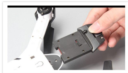
Press slightly to mount/dismount the camera
