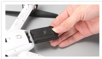
Press slightly to mount/dismount the Battery
